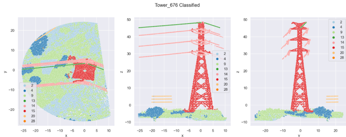
Figure 3: Example of a processed LiDAR transmission tower point cloud
